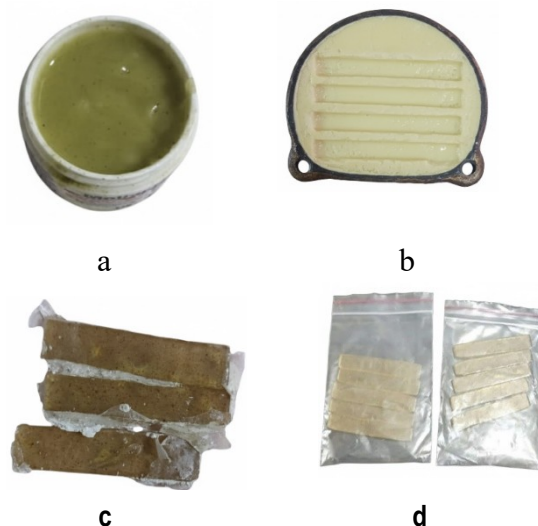
Figure 1: (a) Moringa Powder and Heat Cure Acrylic Powder Mixture (b) Mould Fabrication (c) Un-trimmed and Unfinished samples (d) Final Cured Samples.
